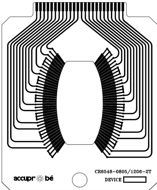
**CR Series** cards are designed for use in the high speed laser trimming of 0805 and 1206 format chip resistors. The cards have been designed to provide high throughput capability for the full range of resistor values. Each card uses an epoxy solder mask to protect the card from Laser trim debris and facilitate easy cleaning. Thick 90 mil stiffeners are bonded to the card to keep the card flat during use and prevent the card from flexing during probe deflection.
