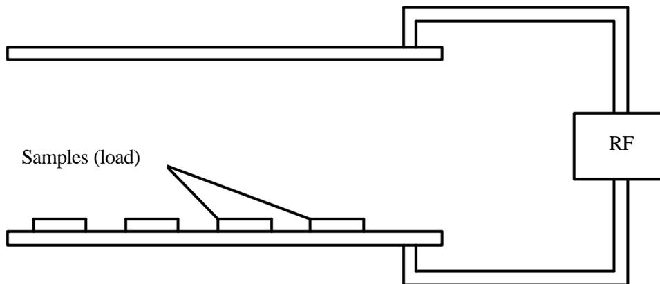
In this methodology, the sample is placed directly onto one of the electrodes. While the parallel plate concept produces a relatively uniform plasma across the sample load, the samples are, by design bombarded with magnetic, RF, electron, x-ray, neutral photon bombardment. Also, thermal energy is unpredictably produced in the workload.
