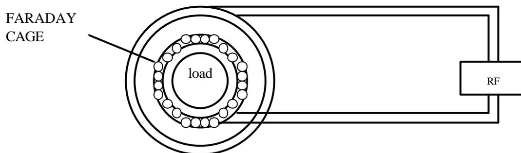
An early design of plasma cleaners involved a design termed a "Barrel" Reactor.
