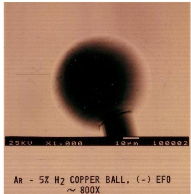
EFO types (positive or negative) were also evaluated by Mitsubishi Wire Company in Japan to better understand its impact in ball shape consistency and concentricity. Their experimental results favored strongly the Positive type EFO as a better method to form consistently shaped free air copper balls.
