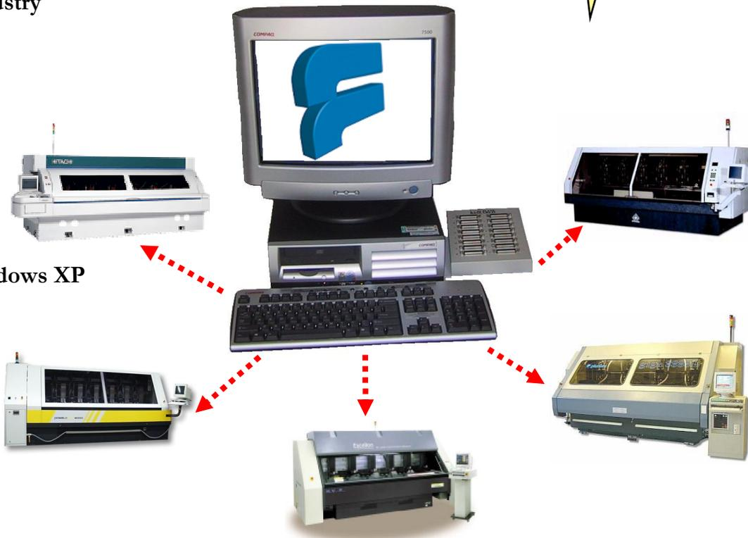
The FASTechnologies DNC UltraServer is a turnkey DNC server based on Microsoft Windows NT/2000/XP. The server comes factory configured and tested, ready to use. UltraServer integrates smoothly with networks running Windows, Novell, and (optionally) NFS network protocols.
